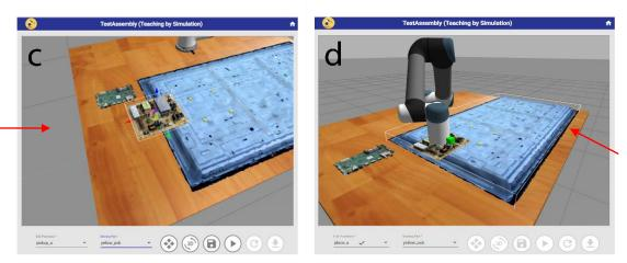
4. User may press the play button to run the simulation and make changes to the keyframes. Assembly process can be exported in JSON file
